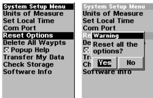
Advanced Mode's Reset Options command, left, and the Reset Options Menu, right.
